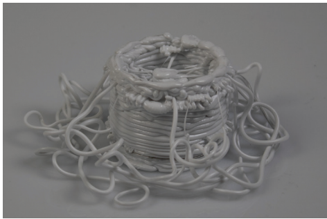
A sample was made, projecting the X-axis outward for a little while and returning to the center, one time looks like an error, repeated makes it look intentional.
