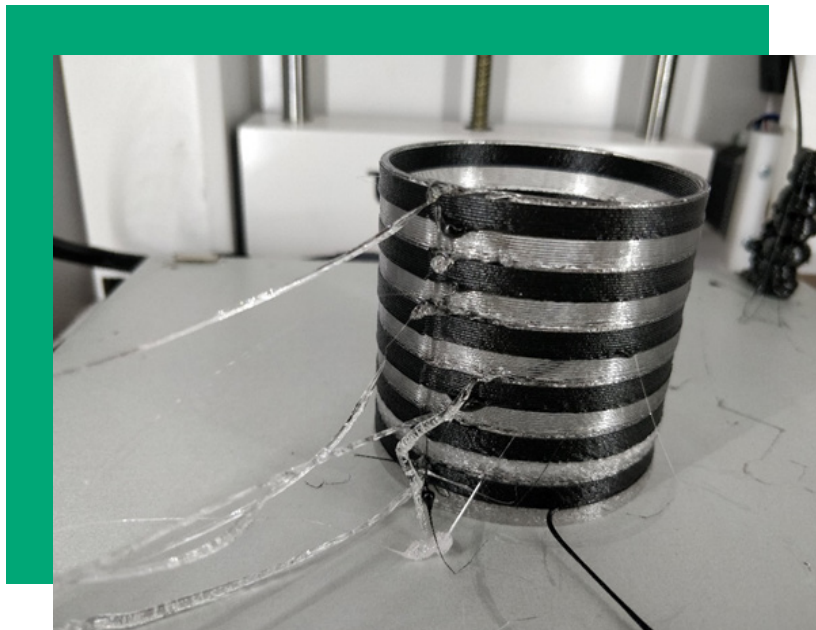
Fig 6; One of the first calibrated prints. It is however evident that drooping needs a remedy.
