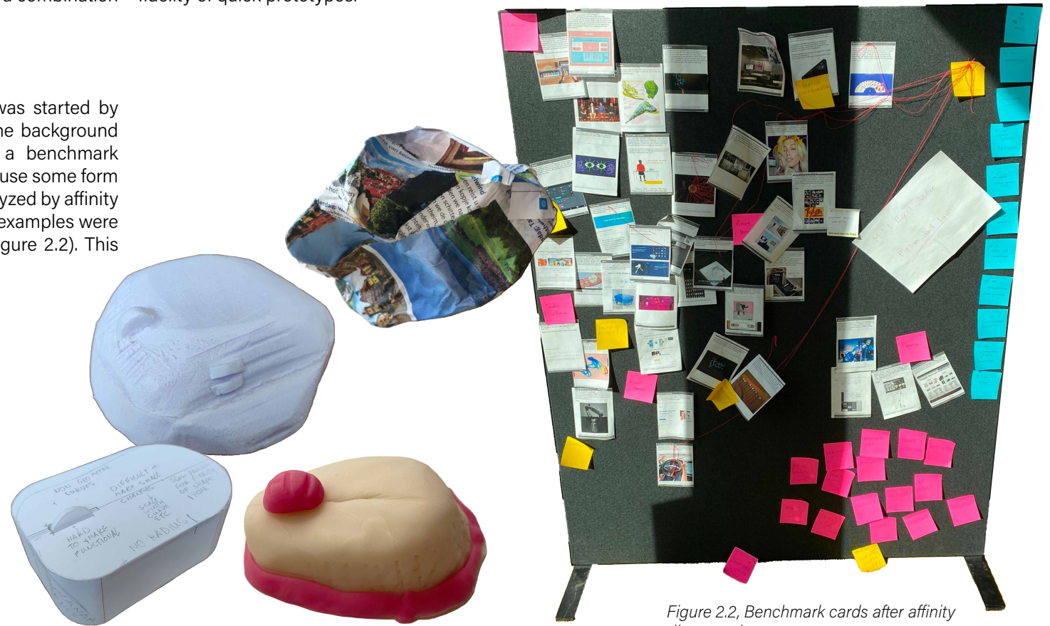
Figure 2.3, Four mouse models. One of styrodur foam, one of papier mache, one of foamboard, and of clay.
