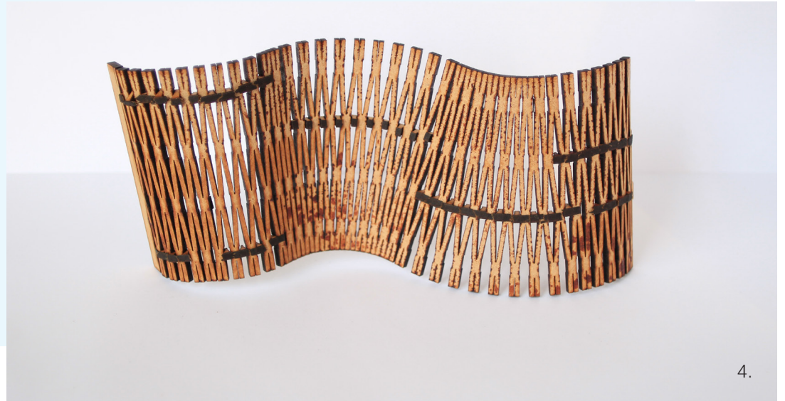
Figure 27, 1 Multicurved surface which cannot be directly calculated with the design editor, 2,3 Jammed 2.5D shape, strips of pins are not possible for assembly, 4 shape memory pins fall out after moving the pattern after a while
